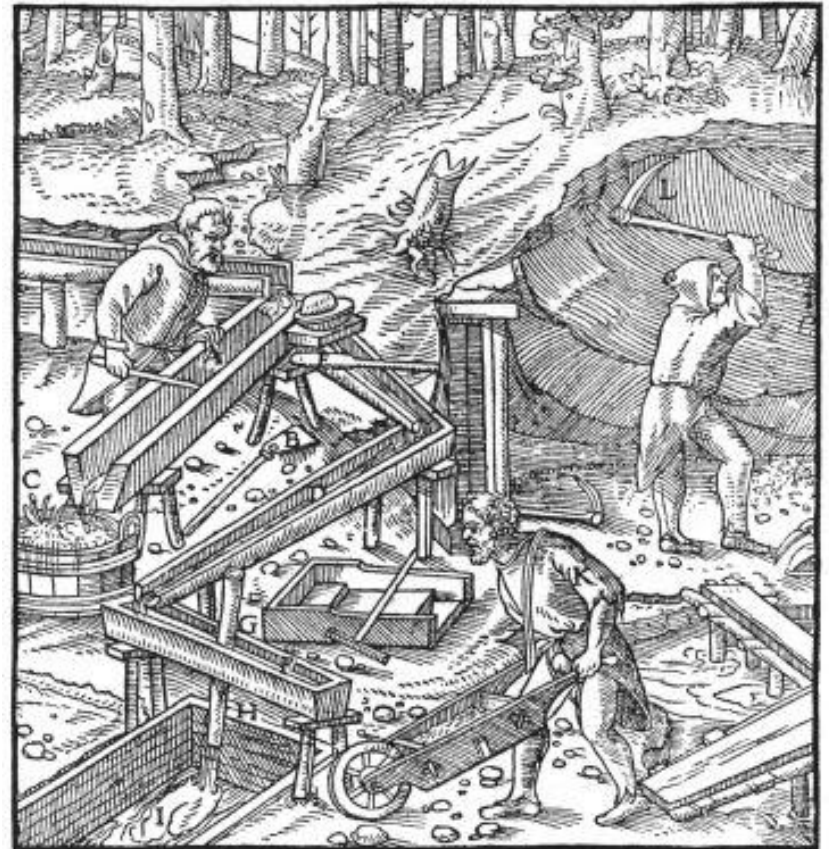
A—TROUGH. B—WOODEN SHOVEL. C—TUB. D—LAUNDER. E—WOODEN TROWEL. F—TRANSVERSE TROUGH. G—PLUG. H—FALLING WATER. I—DITCH. K—BARROW CONVEYING MATERIAL TO BE WASHED. L—PICK LIKE THE BEAK OF A DUCK WITH WHICH THE MINER DIGS OUT THE MATERIAL FROM WHICH THE SMALL STONES ARE OBTAINED.
