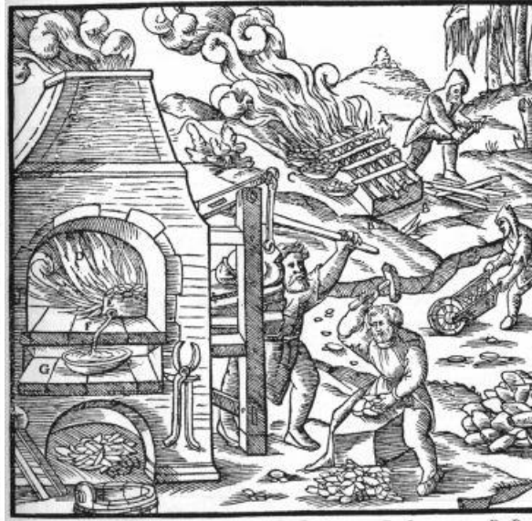
A—WOOD. B—BRICKS. C—PANS. D—FURNACE. E—CRUCIBLE. F—PIPE. G—DIPPING-POT.
